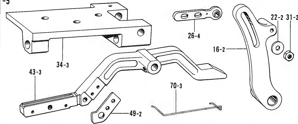
L. 送り関係 (2) / Feed mechanism (2) / Transportvorrichtung (2) /
