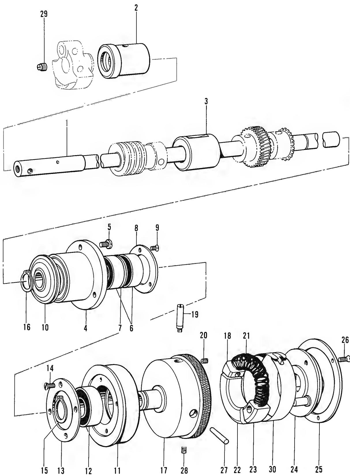
C. 上軸関係 /Upper shaft mechanism/Obere Welle/
