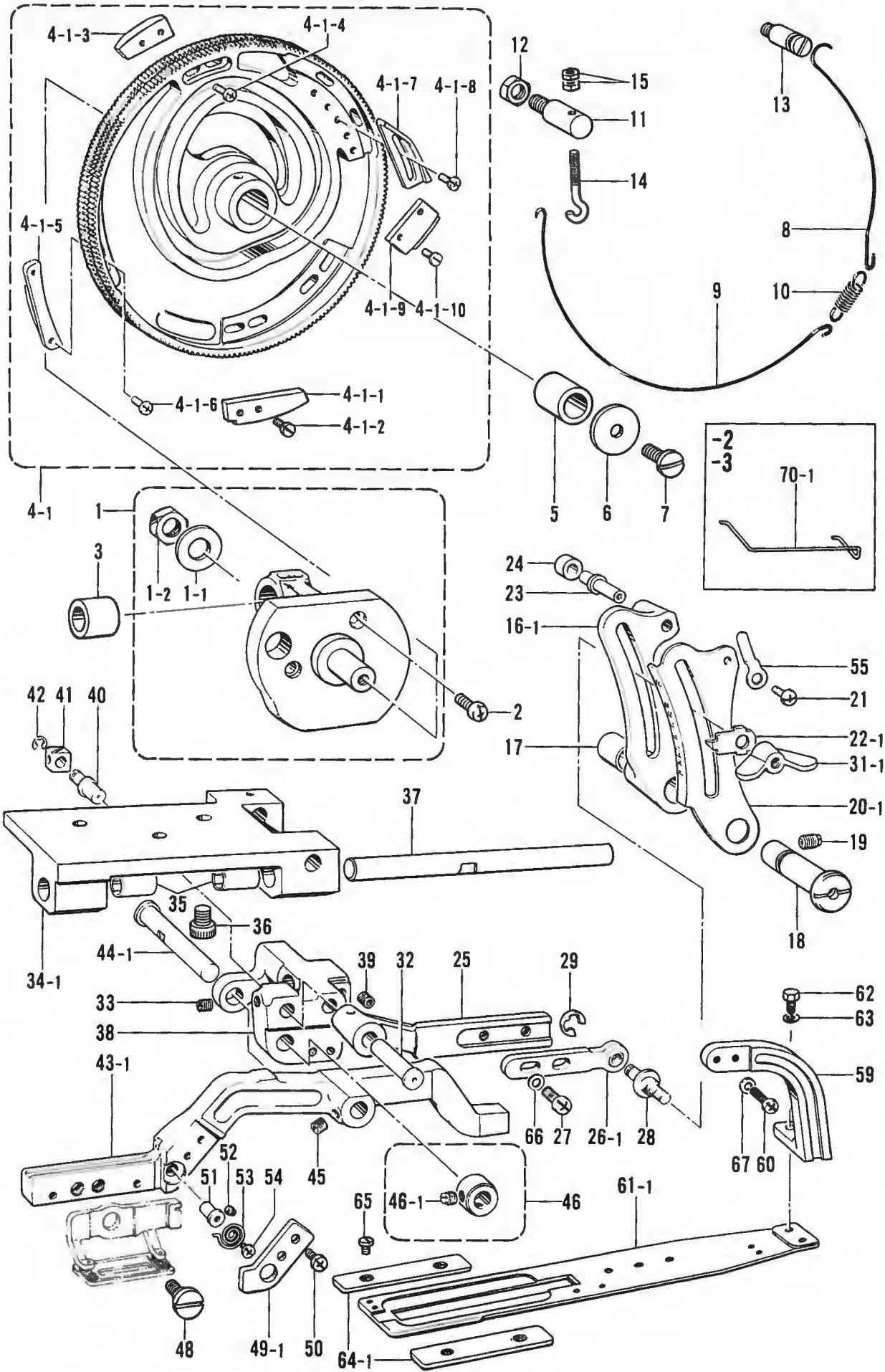
L. 送り関係 (1) /Feed mechanism (1)/Transportvorrichtung (1)/
