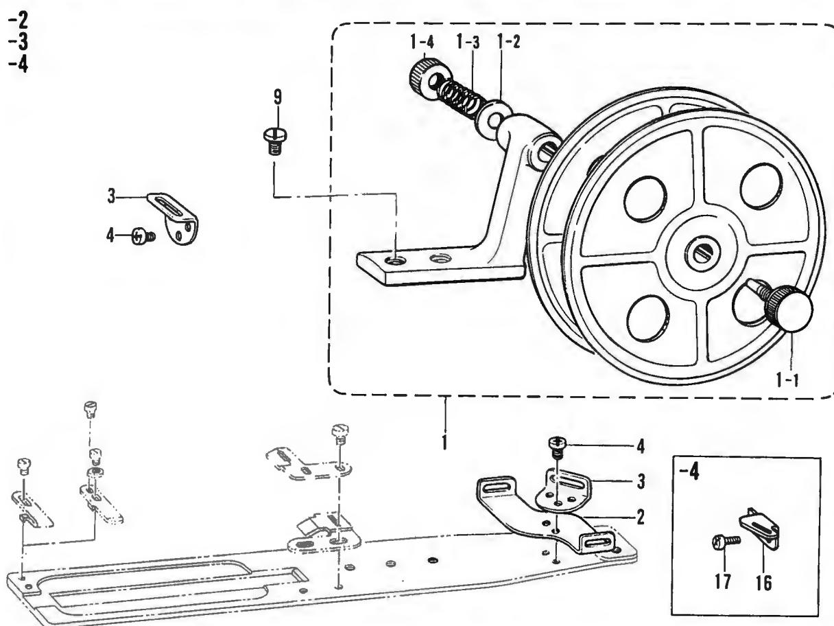
P. 糸切れ感知関係 / Thread breakage detector mechanism / Fadenbruchfühler /
